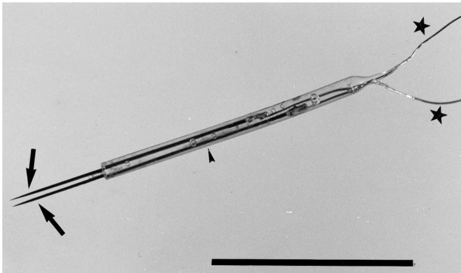
FIG. 1. Photograph showing the floating double microelectrode that has been designed to obtain unitary recordings in neurons in the human spinal dorsal horn. *Arrows* indicate the tungsten-in-glass microelectrodes, glued together in a rigid nylon sleeve (*arrowhead*) filled with silicon rubber. The two independent tips are separated by a distance of 300  $\mu\text{m}$ . *Stars* denote 80- $\mu\text{m}$ -diameter insulated copper connection wires. The electrode weighs 20 mg. Bar = 1 cm.
