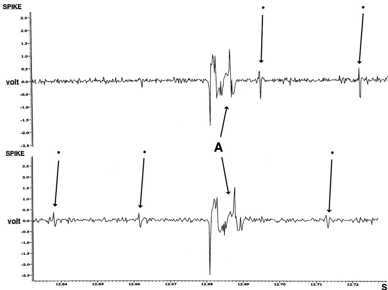
FIG. 5. Example of an easy discrimination between spikes and artifacts generated by the two independent tips. The artifacts (A) are visualized on both channels at the same time, whereas spikes (arrows) are visible only on one channel at a time.
